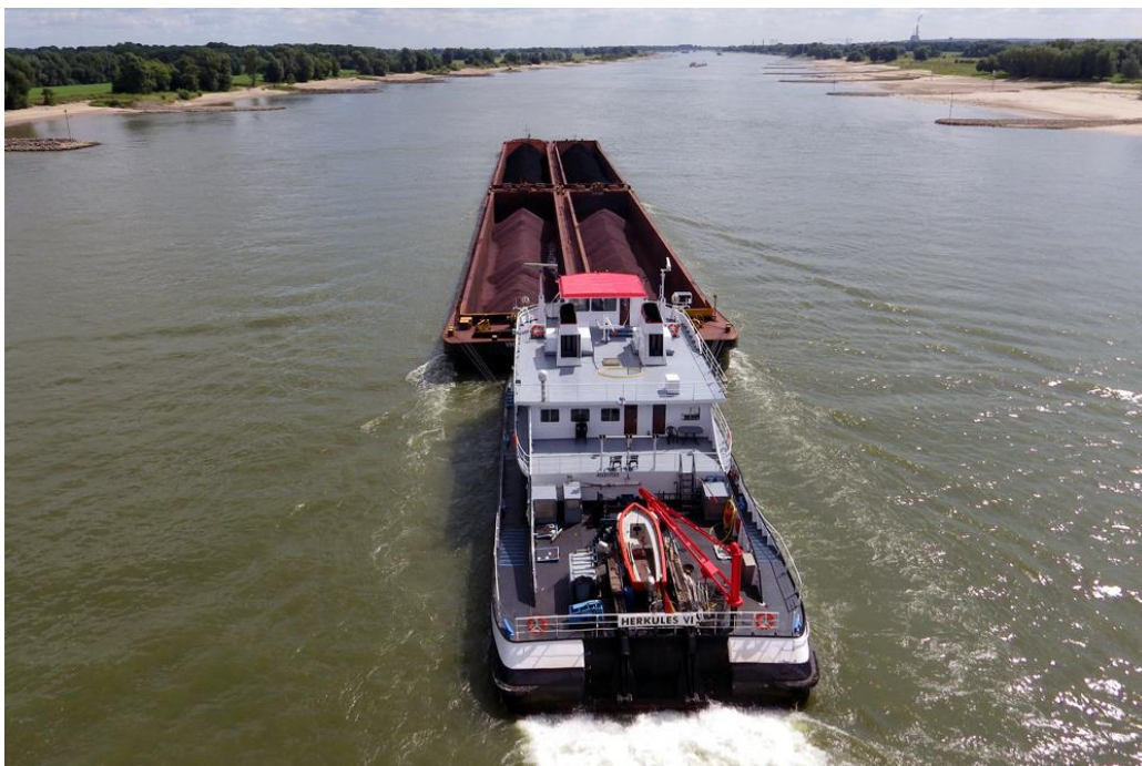
A slightly larger pusher tug heading for the German steel plants pushing four iron ore laden barges.
